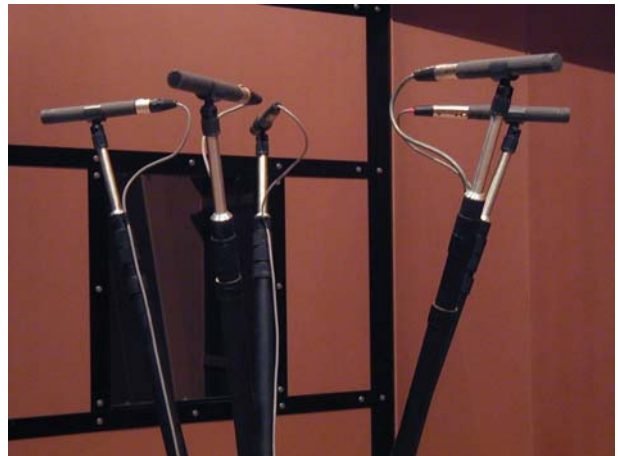
Figure 7 - Microphones adjusted so as to be aligned with the horizontal reference plane
