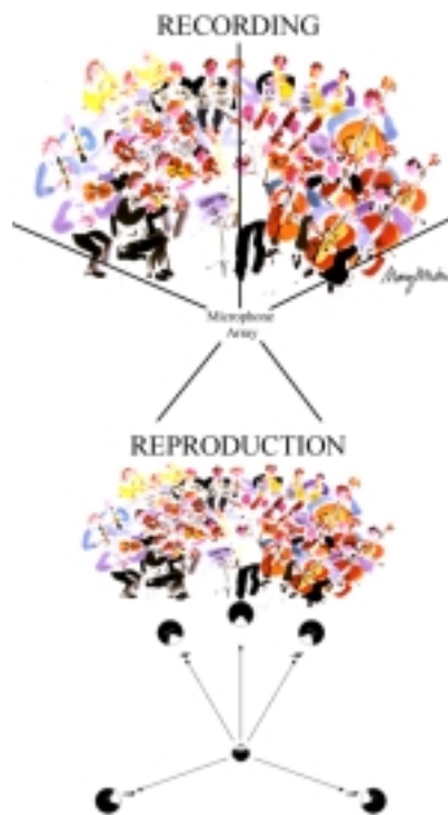
Figure 5 - Front Triplet Coverage is larger than the sound source
